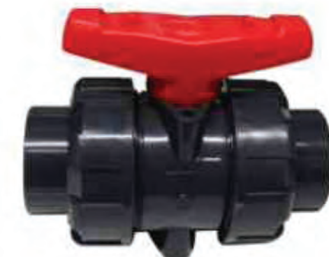
F71 Double Union Ball Valve Size: 1/2" to 4" thread, socket 1/2"-2": 235psi Max. 2-1/2"-4": 150 psi Max.
