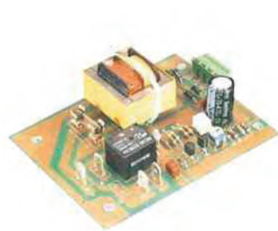
GS-A2016 Sauna controller circuit
