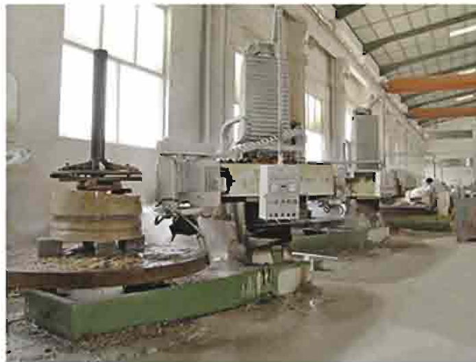
仿型机 Irregular stone process machine
