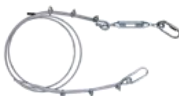
745 - Bracing kit for ceiling suspended goal without pulley. Composed of: Ø6mm Cable, wire thimbles, quick links, cable clamp, turnbuckle (with locking nuts)
