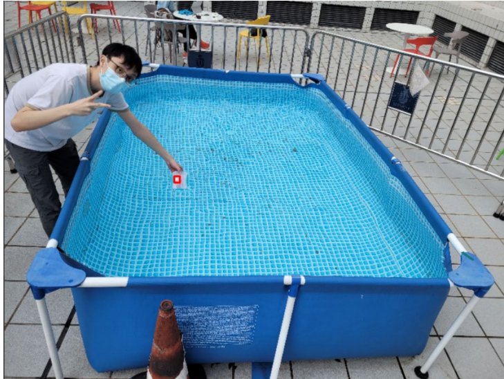
Figure 40 Detected red LED above the water surface at 1m
