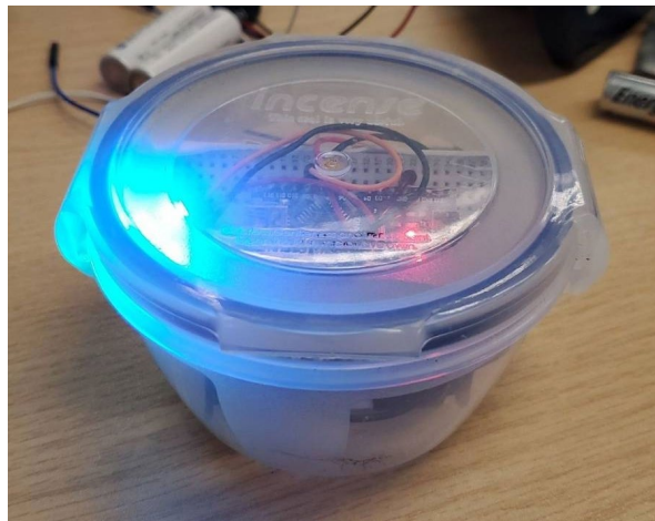
Figure 26 Wearable device placed in the first lock-n-lock box
