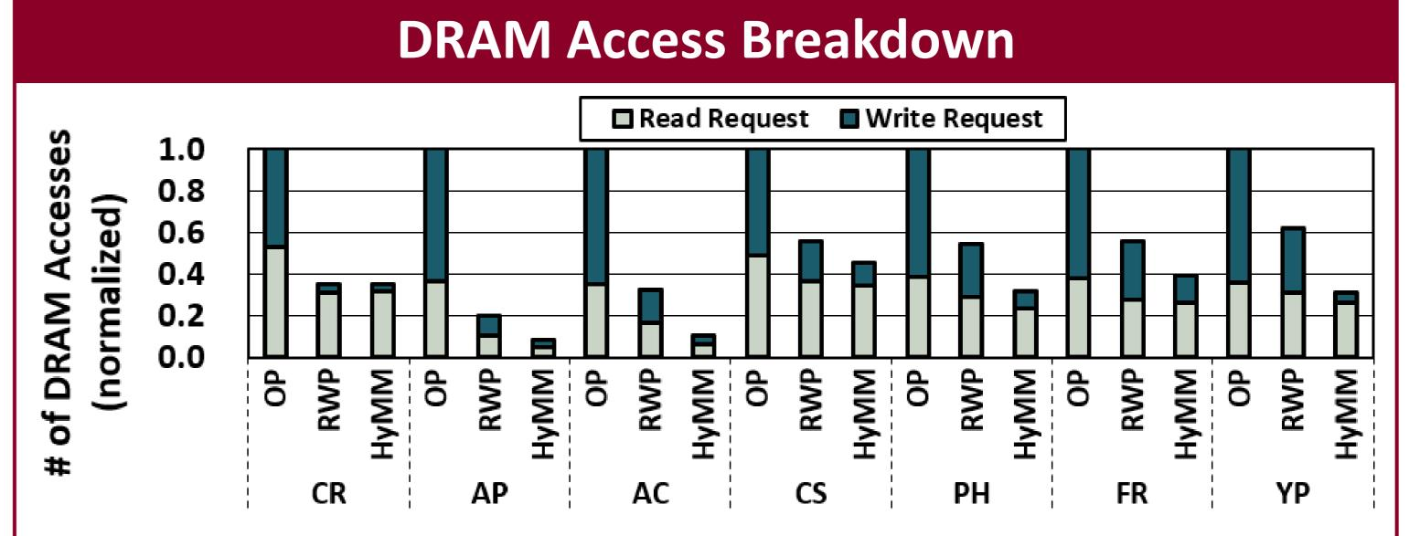
By exploiting data locality efficiently with the hybrid dataflow architecture, **HyMM** can effectively reduce off-chip accesses
