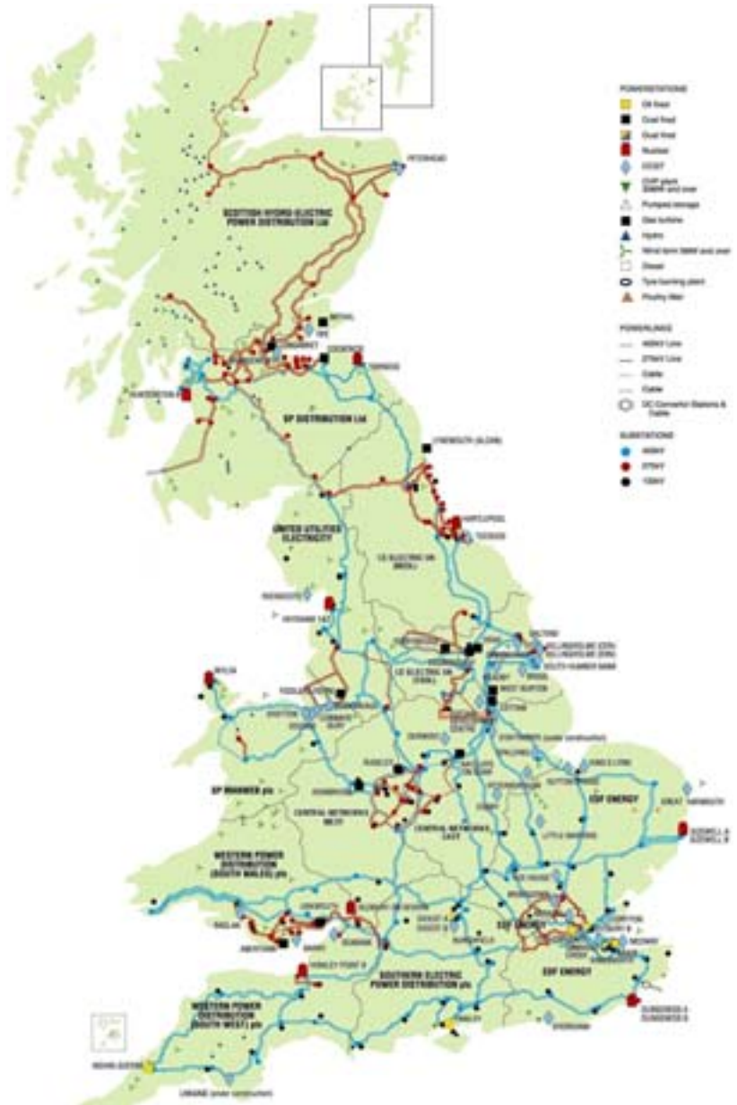
Figure 4-5: The High Voltage Transmission Network in England, Wales and Scotland. The map also indicates the distribution areas and the relevant companies as well as the generation sources/locations.
