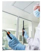
Do you need to carry out measurements in places where Bluetooth isn't possible? No problem: simply switch the probe head over from Bluetooth to the cable handle and you're ready to go.
