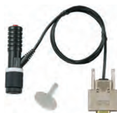
UD-412 Impact device HLDC scale Use for inner walls of cylinders. The grip is short to allow positioning within a cylinder.
