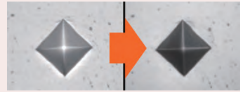
Observation image of the indentation (50X) Stray light reduction around the indentation
