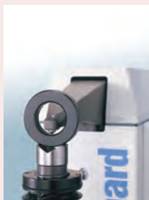
The dolphin-nose indenter arm for inside testing
