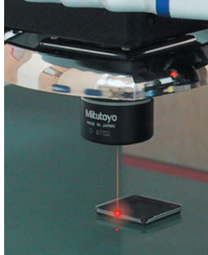
Coaxial laser Tracking Auto Focus (TAF)
