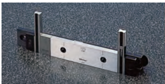
Holder B and C : Used for coupling two long gauge blocks together with other gauge blocks up to 35 mm (Holder B) or 140 mm Holder C). Also used for attaching jaws with two adapters.
