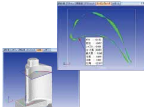
Turbine blade analysis (optional function)
