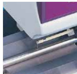
Measuring ball screw
