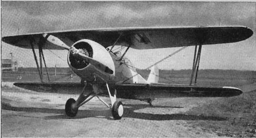
First Vought 200 m.p.h. plane, the SBU-1, had tapered wings, cowl flaps, was built in 1935.
