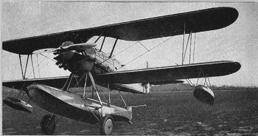
Amphibian landing design made the O3U-1 a versatile multi-purpose plane in 1929.
