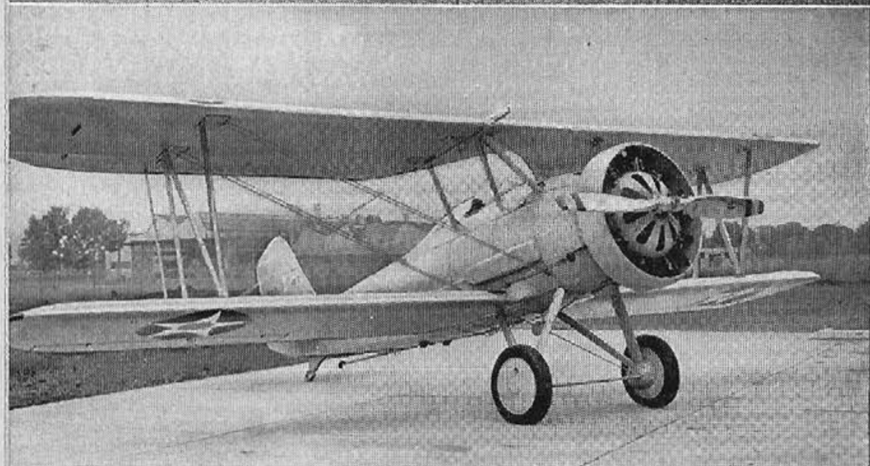
In 1933, a 600 h.p. Hornet engine powered the O3U-2, later designated the SU-1.
