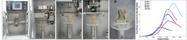
Fig. 6 EPT Test: 1) EPT Tester 2) Confined Consolidation 3) Exposed Sample 4) Unconfined Compression to Failure 5) Failed Sample 6) Typical Measured Stress-Strain Behavior at Various Consolidation Stresses
