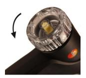
Remove particle filter (1) and store it to reinsert it after the measurement.
