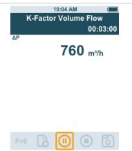
This process for determining volume flow can always be used when there are appropriate specifications available from the component manufacturer. In line with these specifications, the differential pressure is measured at a position specified by the manufacturer or supplier. The volume flow is determined from the differential pressure via a component-specific K-factor using the following mathematical equation:
