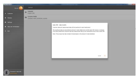
As soon as the testo 400 is connected via a USB cable to a computer, Connected to testo 400 – Synchronizing is displayed at bottom left. A message about data transfer is displayed. Confirm by pressing OK to transfer all customer and measurement data from the testo 400 to the software. The
