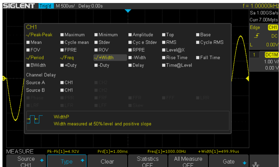
Figure 88 Select the Measurement Parameter
