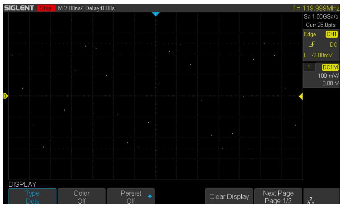
Figure 16 Display Type Set to Dots
