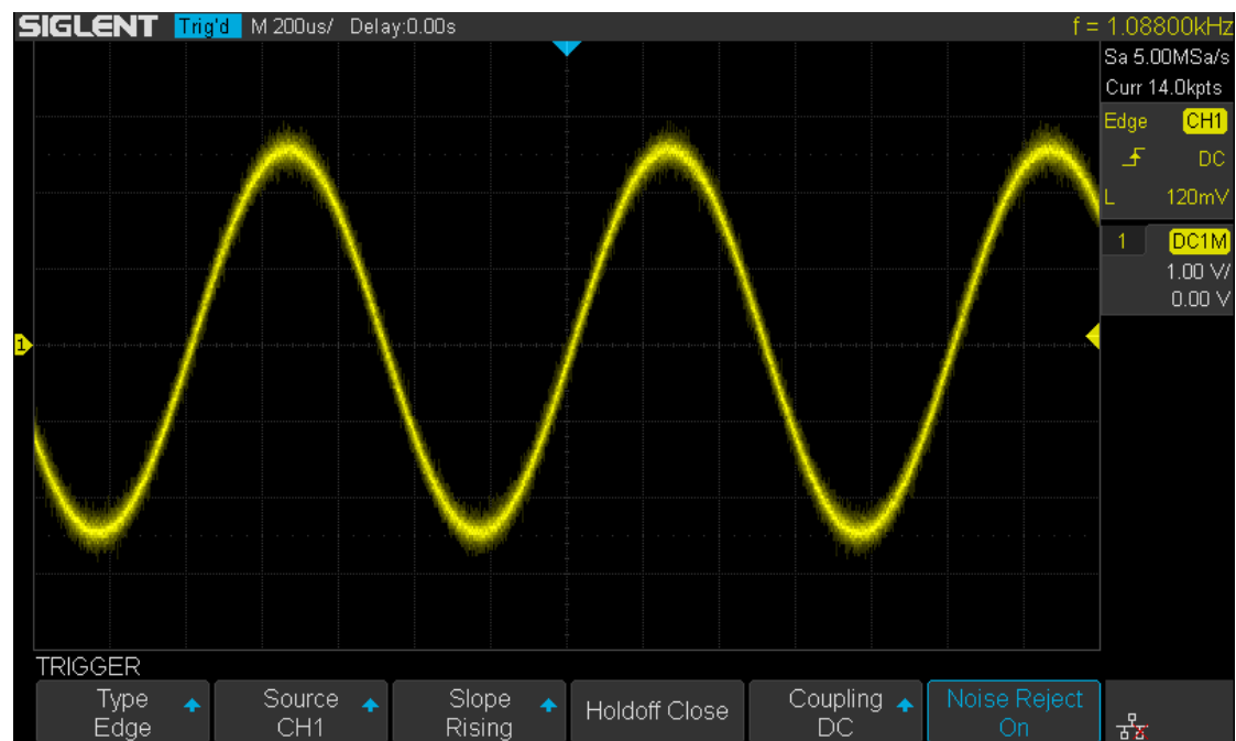
Figure 27 Turn on the Noise Reject
