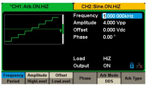
Figure 2-18 Arb Parameters Display Interface (DDS)
