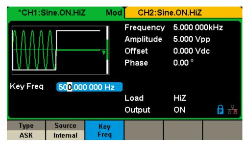
Figure 3-13 Generate an ASK Modulation Waveform
