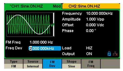
Figure 3-10 Generate a FM Modulation Waveform
