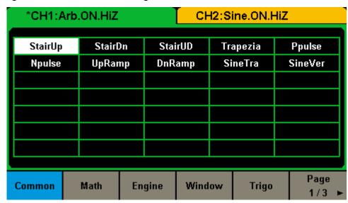
Figure 2-21 Built-in Arbitrary Waveforms
