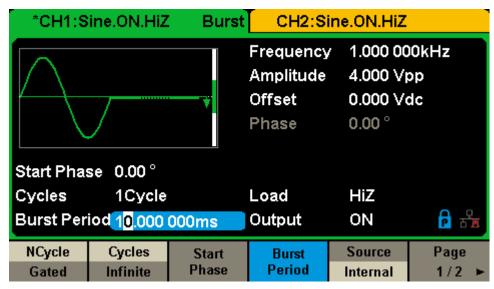
Figure 1-16 Burst Waveform Display Interface
