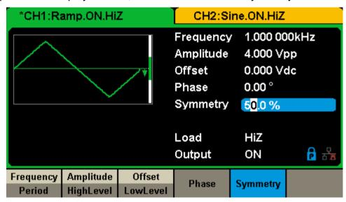
Figure 2-8 Ramp Parameters Display Interface
