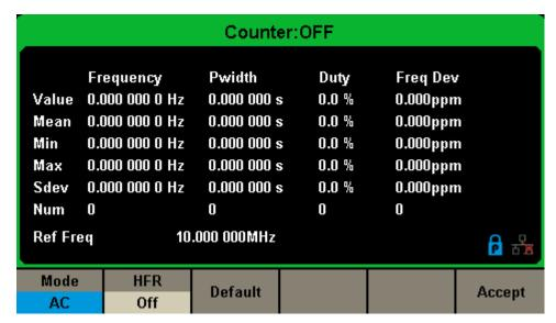
Figure 2-65 Counter Setup Interface
