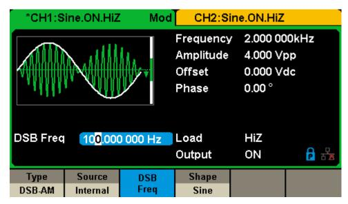
Figure 3-16 Generate a DSB-AM Modulation Waveform
