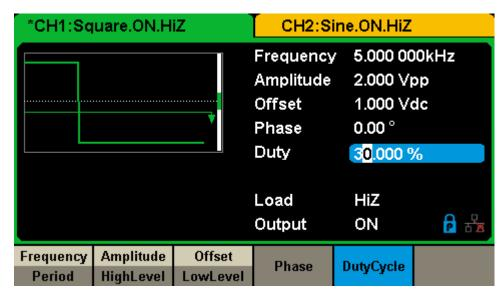
Figure 3-2 Generate a Square Waveform
