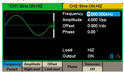
Figure 2-1 Sine Parameters Display Interface
