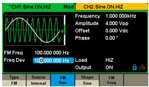
Figure 2-26 Setting Interface of FM Modulation
