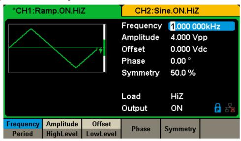
Figure 1-8 Ramp Display Interface
