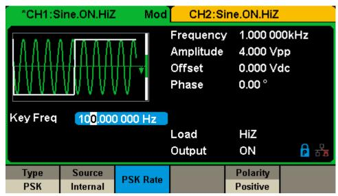
Figure 2-30 Setting Interface of PSK Modulation
