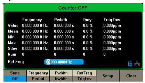
Figure 2-64 Frequency Counter Interface
