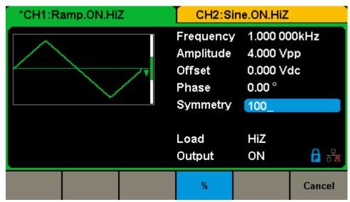
Figure 2-9 Setting the Symmetry
