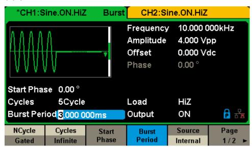
Figure 3-8 Generate a N-Cycle Burst Waveform
