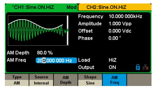
Figure 3-9 Generate an AM Modulation Waveform
