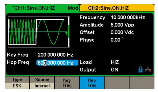
Figure 3-12 Generate a FSK Modulation Waveform
