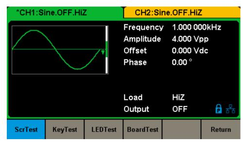
Figure 2-57 Self Test Interface
