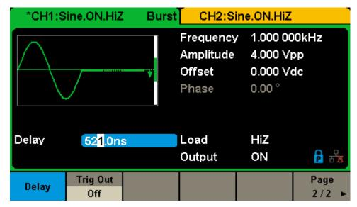
Figure 2-39 N-Cycle Burst Interface (Page 2/2)
