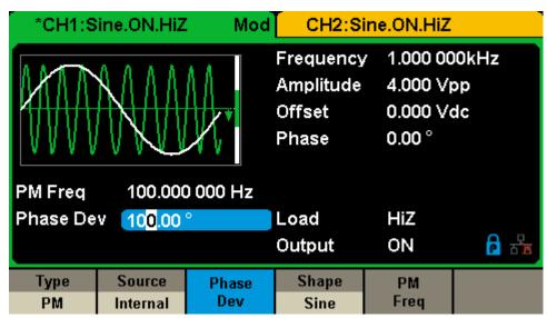
Figure 2-27 Setting Interface of PM Modulation
