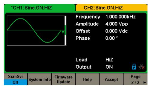
Figure 2-49 System Setup Interface (Page 2/2)
