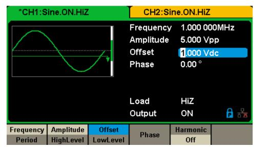
Figure 3-1 Generate a Sine Waveform
