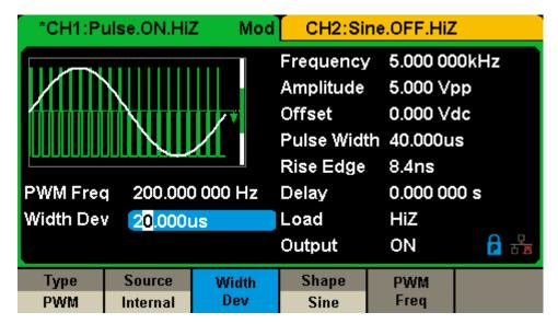
Figure 3-15 Generate a PWM Modulation Waveform
