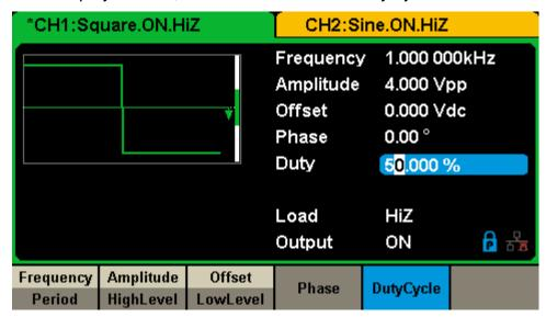
Figure 2-6 Square Parameters Display Interface
