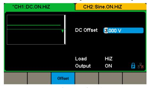
Figure 3-6 Generate a DC Waveform
