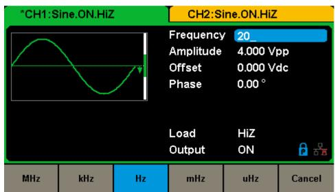
Figure 2-2 Setting the Frequency
