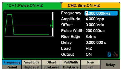
a pulse waveform with different parameters can be generated.
