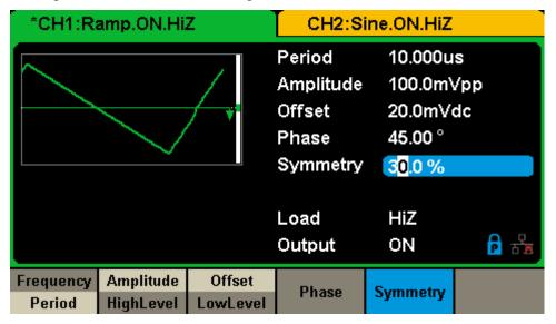
Figure 3-3 Generate a Ramp Waveform
