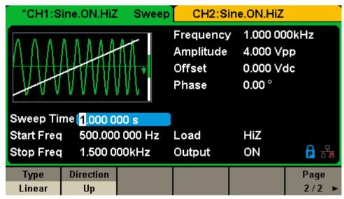
Figure 2-36 Linear Sweep Interface
