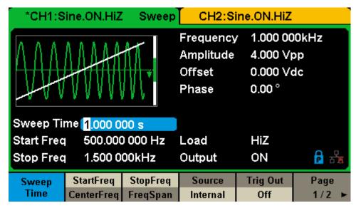
Figure 1-15 Sweep Waveform Display Interface
