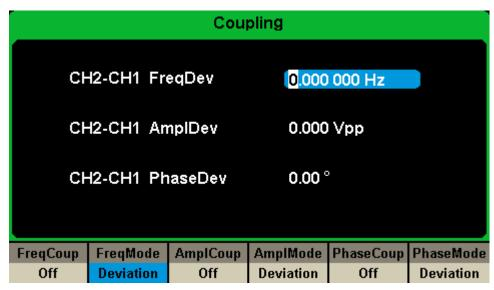
Figure 2-69 Channel Coupling Interface
