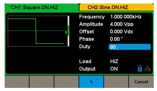
Figure 2-7 Setting the Duty Cycle
