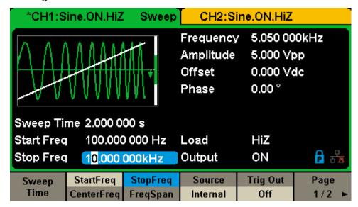
Figure 3-7 Generate a Linear Sweep Waveform
