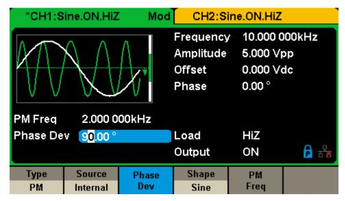
Figure 3-11 Generate a PM Modulation Waveform
