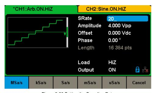
Figure 2-20 Setting the Sampling Rate
