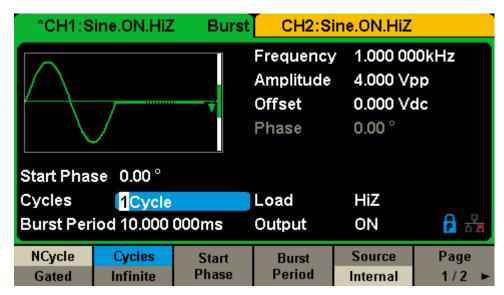
Figure 2-38 N-Cycle Burst Interface (Page 1/2)
