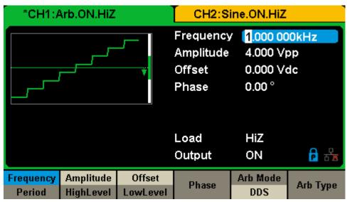
Figure 1-12 Arbitrary Waveform Display Interface
