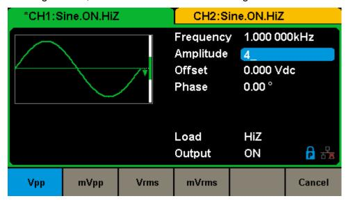
Figure 2-3 Setting the Amplitude
