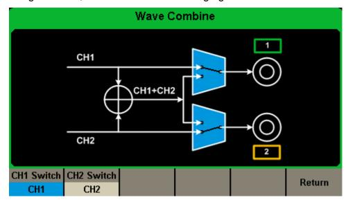
Figure 2-67 Waveforms Combining Interface
