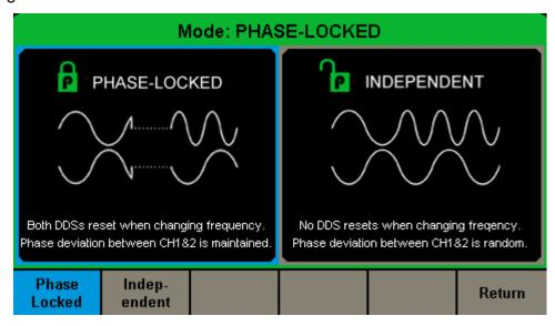
Figure 2-76 Mode Setup Interface
