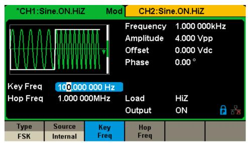
Figure 2-28 Setting Interface of FSK Modulation
