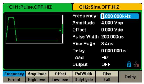
Figure 2-10 Pulse Parameters Display Interface
