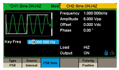
Figure 3-14 Generate a PSK Modulation Waveform
