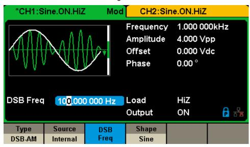
Figure 2-25 Setting Interface of DSB-AM Modulation
