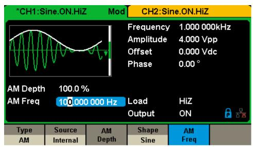
Figure 2-24 Setting Interface of AM Modulation
