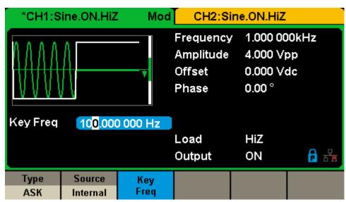
Figure 2-29 Setting Interface of ASK Modulation
