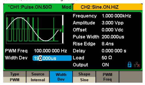
Figure 2-32 Width Deviation Setting Interface
