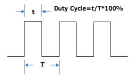
The duty cycle setting range is limited by the "Frequency/Period" setting. For detailed information, please refer to "SDG2000X Datasheet". The default value is 50%.
