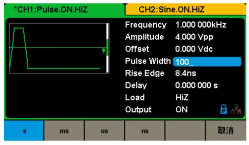
Figure 2-11 Setting the Pulse Width
