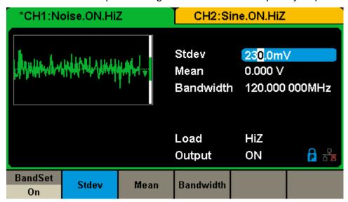
Figure 2-13 Noise Parameters Display Interface
