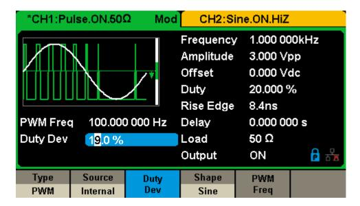
Figure 2-33 Duty Deviation Setting Interface
