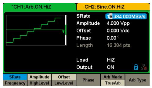
Figure 2-19 Arb Parameters Display Interface (TrueArb)
