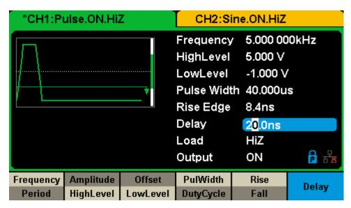
Figure 3-4 Generate a Pulse Waveform
