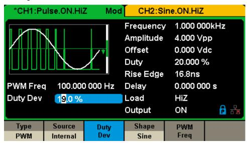
Figure 2-31 Setting Interface of PWM Modulation
