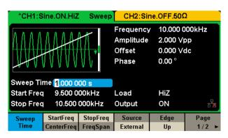
Two Sweep modes, "Linear" and "Log". Two Sweep directions, "Up" and "Down" and three Sweep sources, "Internal", "External" and "Manual".
