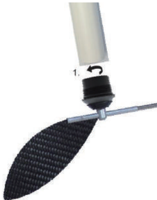
Figure 9.( Bearing replacement – Wind speed/direction sensor)
