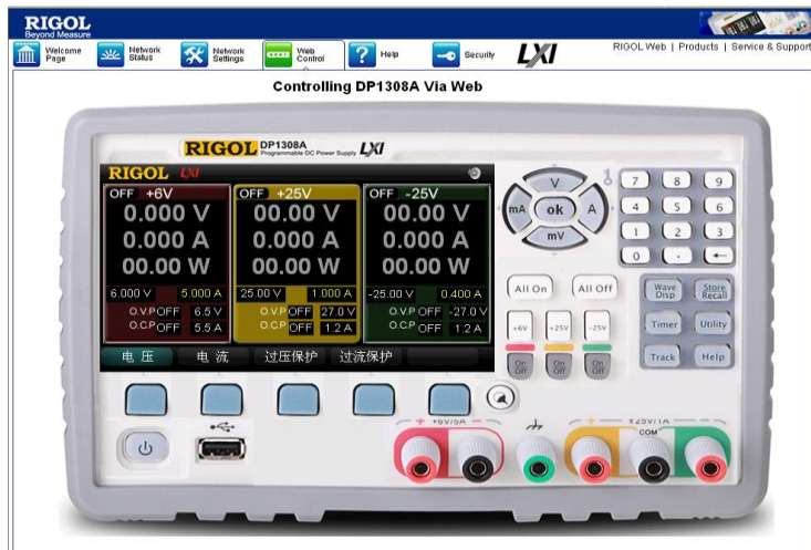
Figure 3-5 Control DP1308A via web
