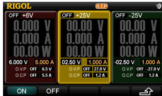
Figure 2-28 Over-temperature Protection Settings
