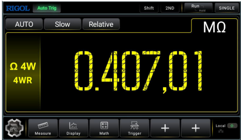
Figure 5.13 4WR Measurement Interface
