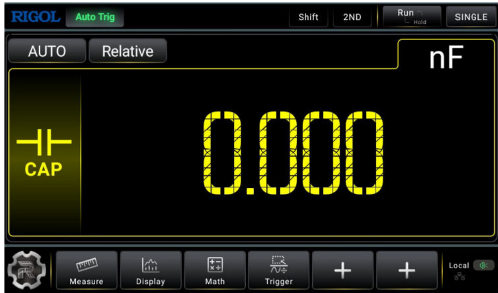
Figure 5.15 Capacitance Measurement Setting Interface
