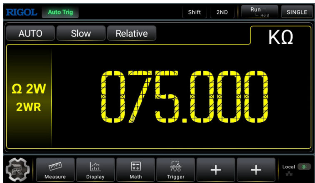
Figure 5.11 2WR Measurement Interface
