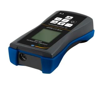
Coating thickness gauge with V-groove sensor / Measuring range from up to 0 ... 5000  $\mu$ m / Adjustable alarm limits / Robust housing / Software / Data storage / High accuracy of up to  $\pm (1.0\%$  of reading + 0.5  $\mu$ m) / Optionally with ISO calibration certificate
