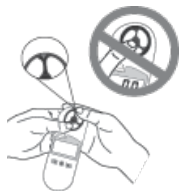
Replacing the Impeller
