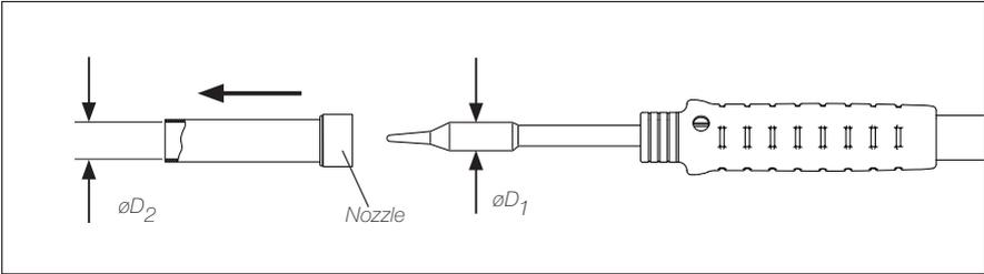
If the outer cartridge diameter  $D_1$  is larger than the inner nozzle diameter  $D_2$ , The cartridges must be removed first before the nozzle can be removed.
