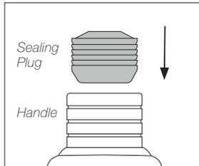
**Note:** The chamfered side has to be positioned towards the handle.
