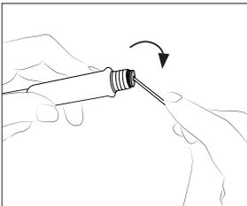
Enter, not deeper than 8mm, a small shaft or screwdriver, lift and pull the sealing plug. Never use a cartridge to do this operation.
