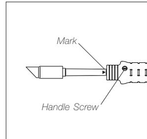
**Note:** After proper cartridge insertion as far as the mark
