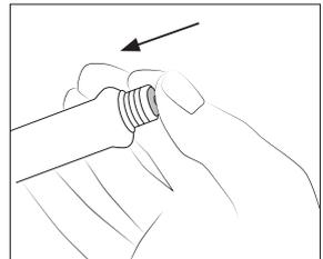
Push the sealing plug inside the handle until the sealing plug and handle edges are aligned.
