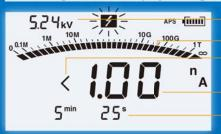
Actual output voltage Resistance value < flashes when less than 1 nA
