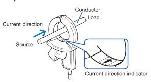
If the clamp is attached with the current direction indicator pointed in the opposite direction of the current, the phase is displayed deviating by 180 degrees.
