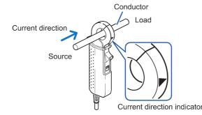
If attached with the current direction indicator pointed in the opposite direction of the current, the phase is displayed deviating by 180 degrees. 5 Make sure the jaw is firmly closed.
