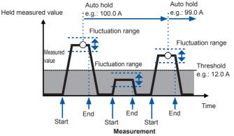
If the measured value falls below the threshold value (voltage, current) or exceeds the threshold value (resistance, continuity, diode) after display value updates are stopped, the display value update is restarted. Display value updates will stop if the two conditions are satisfied once again.
