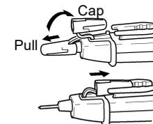
When using the 3246, remove the cap and securely fasten the cap to the rear, as shown in the figure.
