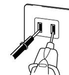
2. Connect the test leads to the measurement object, and read the indicated value.
