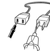
2. Connect the test leads to the measurement object. When the continuity (threshold: 50±40  $\Omega$  or less) is established, the beeping sounds.
