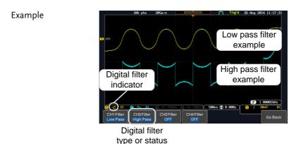
CH1 input: 2Vpp 1kHz square wave, low pass filter with 1kHz cutoff frequency.
