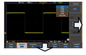
1. Press the *Menu Off* key to reduce the side menu, press again to reduce the bottom menu.
