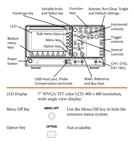
Menu Keys The side menu and bottom menu keys are used to make selections from the soft-menus on the LCD user interface.
