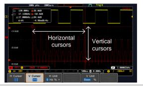
XY Mode XY mode cursors measure a number of X by Y measurements.
