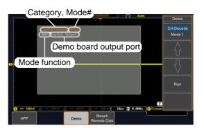
As shown above, the demo category, mode number, mode function and the relevant demo board output ports are shown on the pop-up window.
