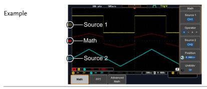
Position and Unit To move the math waveform vertically, press the *Position* key from the side menu and use the *Variable* knob to set the position.
