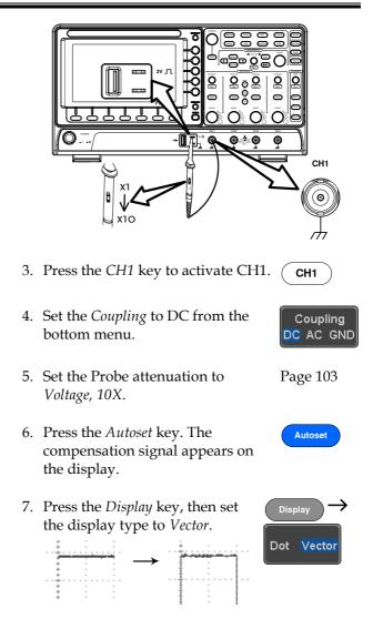
8. Turn the adjustment point on the probe to make the waveform as square as possible.
