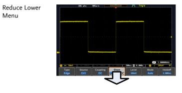
1. Press the relevant function key again to reduce the bottom menu. For example: press the Trigger Menu key to reduce the trigger menu.
