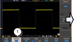
1. To reduce the side menu, press the corresponding bottom menu that brought up the side menu originally.
