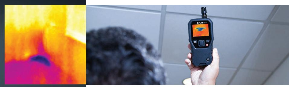
Featuring IGM technology powered by a built-in thermal imaging sensor, the MR176 and MR160 can visually guide you to the precise spot that moisture may be hiding
