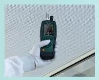
The VPC260 is a 6-channel particle counter for monitoring workplace environmental health and air quality. Measure up to 6 channels of particle sizes plus air temperature, relative humidity, dew point, and wet bulb. Check for harmful air pollutants such as exhaust, smoke, respirable crystalline silica dust (RCS), and airborne combustible dust once particles are detected.
