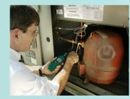
Compact meter is well-suited for field applications. Unique sensor cap closes for protection during storage. Simultaneously displays relative humidity, air temperature and dew point or wet bulb. Calculates T1-T2 differential (air temperature minus external probe temperature) using optional probe (TP890), and T2 minus dew point. Other features include Data Hold, Auto Power Off, and MAX/MIN reading.
