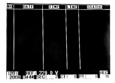
NOTE: Each time the  $1\Phi$   $3\Phi$  button is pressed, the meter steps through the transient mode wire configuration list (1P2W, 1P3W, 3P3W, and 3P4W)
