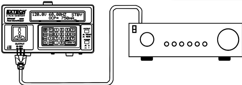
Connect the Unit Under Test to the 380820.
