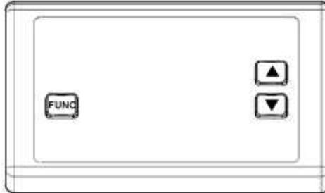
1. The LCD displays the power data of the Rear Output.
