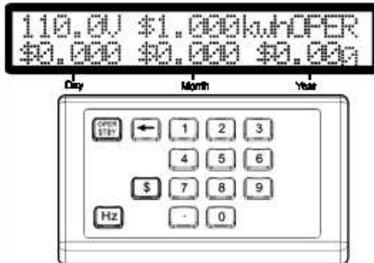
1. Program the power cost per KWh and press the \$ button.
