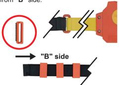
3. Turn over the elastic cord and take the elastic cord adjustment pass through from "B" side.
