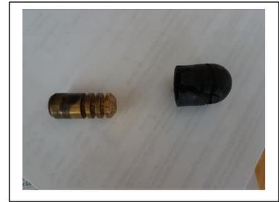
The cause is internal corrosion of the steel rod and galvanized pipe. Rust is produced and it has restricted the movement of the rubber plug and/or rod itself. It has even eaten right through the steel rod and/or galvanized pipe. It appears that the hydrants that are shut off for the winter, combined with the fact that the water table prevents proper draining, may result in hydrants that are in worse shape.
