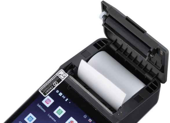
(Figure 2- 4) Install the printer paper
