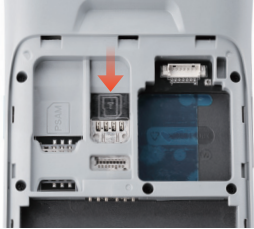
(Figure 2- 2) Insert SIM card
