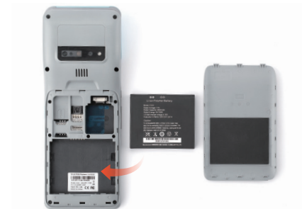
(Figure 2-1) Battery Installation
