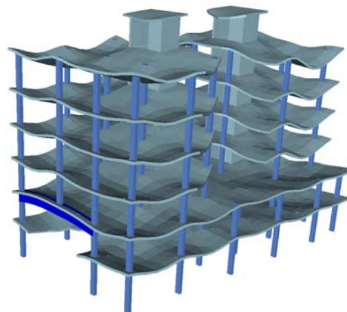
Building model showing global deflected shape from integrated analysis results
