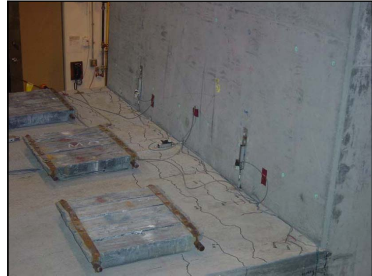
View of full-size post-tensioned slab with core wall and column connection under test
