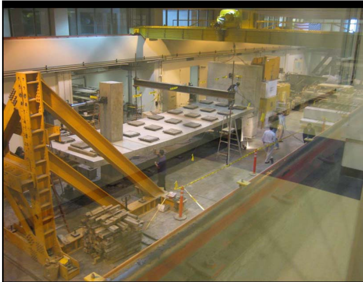
View of full-size test of post-tensioned slab with core wall and column connection
