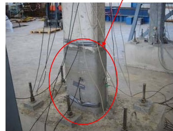
Tested at 0.3g before retrofitting Video 6
