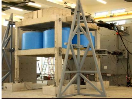
Tested at 0.3g before retrofitting Video 6
