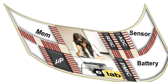
Figure 1: An illustration of flexible hybrid electronics system with flexible circuits, display, battery and rigid CMOS ICs.
