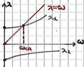
$\Rightarrow$  ONE CRITICAL SPEED :  $\frac{I_p}{I_d} < 1$  ;  $\omega_{CR} = \sqrt{\frac{K}{I_d - I_p}}$
