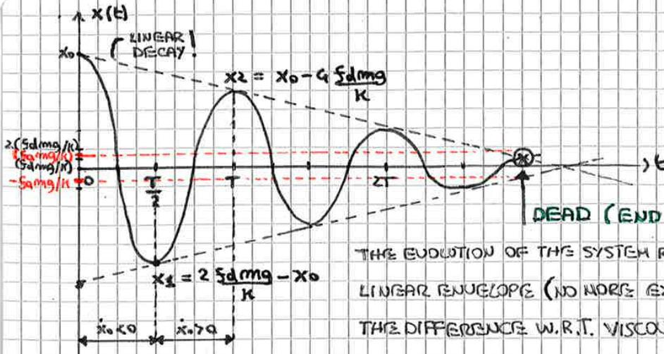
THE EVOLUTION OF THE SYSTEM RESPONSE IS DESTROYED BY A LINEAR ENVELOPE (NO MORE EXPONENTIAL ONE). THIS IS THE DIFFERENCE W.R.T. VISCOUS SYSTEMS (EXP. ENVELOPE)!
