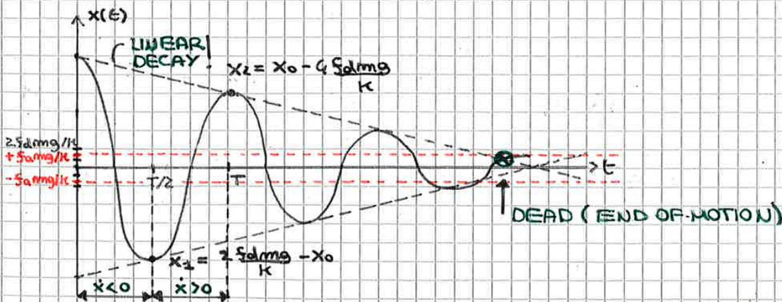
THE MOTION IS STOPPED WHEN  $|x_0 - 2m \frac{f_d mg}{K}| \leq \frac{f_d mg}{K}$  ,  $m = n$  OF HALF-CYCLES
