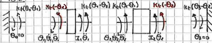
$$1) I_1 \ddot{\theta}_1 + k(\theta_1 - \theta_2) = -k\theta_1 \iff I_1 \ddot{\theta}_1 + 2k\theta_1 - k\theta_2 = 0 \quad \begin{bmatrix} I_1 & \\ & I_2 \end{bmatrix} \begin{bmatrix} \ddot{\theta}_1 \\ \ddot{\theta}_2 \end{bmatrix} + \begin{bmatrix} 2k & -k \\ -k & 2k \end{bmatrix} \begin{bmatrix} \theta_1 \\ \theta_2 \end{bmatrix} = \begin{bmatrix} 0 \\ 0 \end{bmatrix}$$
