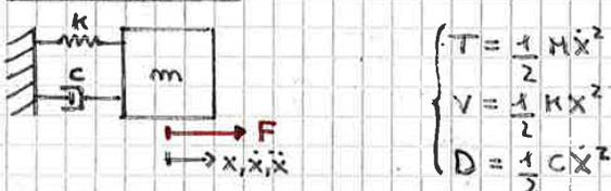
$$\frac{d}{dt} \left( \frac{\partial L}{\partial \dot{q}_k} \right) - \frac{\partial L}{\partial q_k} = Q_k \quad (\Leftrightarrow) \quad M \ddot{x} + Kx = Q_k$$
