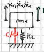
$$m_1 \ddot{x}_1 + k_1 x_1 = F(t) = F_0 \cos(\omega t) = F_0 e^{i\omega t}$$
