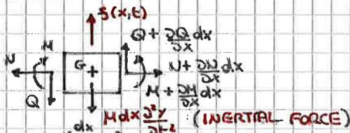
$$\uparrow \sum F_y = 0 \Rightarrow Q + \frac{\partial Q}{\partial x} dx - Q + f(x, t) dx - M dx \frac{\partial^2 y}{\partial t^2} = 0 \quad (0 \leq x \leq L)$$
