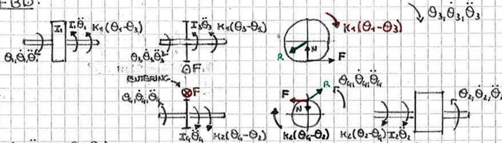
$$\begin{cases} I_1 \ddot{\theta}_1 + k_1(\theta_1 - \theta_3) = 0 \\ I_3 \ddot{\theta}_3 + k_1(\theta_3 - \theta_1) + FR_3 = 0 \quad \leftrightarrow \quad I_3 \ddot{\theta}_3 + FR_3 = k_1(\theta_1 - \theta_3) \\ I_4 \ddot{\theta}_4 + k_2(\theta_4 - \theta_2) - FR_4 = 0 \quad \leftrightarrow \quad I_4 \ddot{\theta}_4 + k_2(\theta_4 - \theta_2) = FR_4 \\ I_2 \ddot{\theta}_2 + k_2(\theta_2 - \theta_4) = 0 \end{cases}$$
