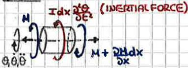
$$\sum \tau = 0 \Rightarrow -M + M + \frac{\partial M}{\partial x} dx - I dx \frac{d^2 \theta}{dt^2} = 0 \quad \text{WITH } I : \text{ MASS MOMENT PER UNIT LENGTH } [\text{kg} \cdot \text{m}^2 / \text{m}] = [\text{kg} \cdot \text{m}]$$
