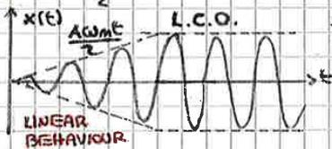
SOMETHING (NATURE OF SYST./FAILURE) STOPS THE AMPLITUDE INCREASING
