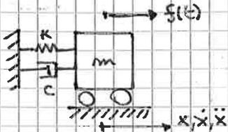
$m\ddot{x} + c\dot{x} + kx = f(t)$  (IN A CYCLE) /  $m\ddot{x}, kx$  ARE CONSERVATIVE  $\Rightarrow$  AFTER A C. THEY ARE NE 0
