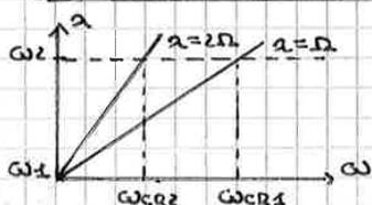
$\Omega_{ENG} = K \left( \frac{2 \cdot m_{cyl}}{m_{st}} \right) \omega_{cr2}, \quad \omega = \frac{2\pi M}{60} \quad (\pi = 3.1416)$
