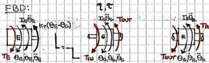
$$\eta = \frac{P_{OUT}}{P_{IN}} ; \quad \tau = \frac{W_{OUT}}{W_{IN}} = \frac{\dot{\theta}_{OUT}}{\dot{\theta}_{IN}} = \frac{\theta_R}{\theta_E}$$
