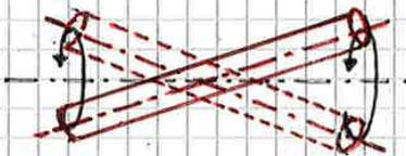
**- FLEXIBLE SHAFT ON RIGID BEARINGS (← JEFFCOTT MODEL)**
