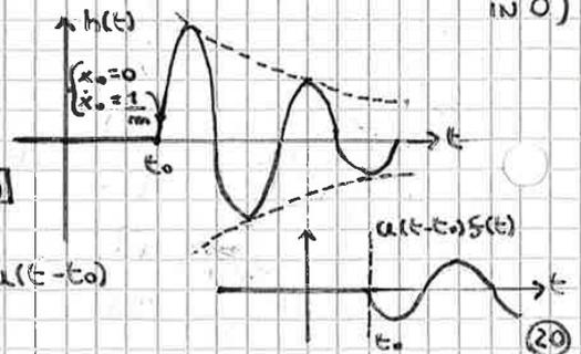
$\begin{cases} u(t-t_0) = 0 \text{ FOR } t < t_0 \Rightarrow x(t) = 0 \\ u(t-t_0) = 1 \text{ FOR } t > t_0 \Rightarrow x(t) = \frac{1}{m \omega_d} e^{-\zeta \omega_n (t-t_0)} \sin[\omega_d (t-t_0)] \end{cases}$
