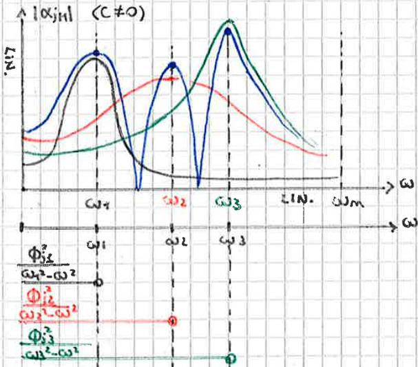
$$\alpha_{jj}(\omega) = \sum_{R=1}^3 \frac{\Phi_{jR}^2}{\omega_R^2 + 2i zeta_R \omega_R \omega - \omega^2} = \sum_{R=1}^3 \frac{\Phi_{jR}^2}{\omega_R^2 - \omega^2} = \frac{\Phi_{j1}^2}{\omega_1^2 - \omega^2} + \frac{\Phi_{j2}^2}{\omega_2^2 - \omega^2} + \frac{\Phi_{j3}^2}{\omega_3^2 - \omega^2} + \dots + \frac{\Phi_{jm}^2}{\omega_m^2 - \omega^2}$$
