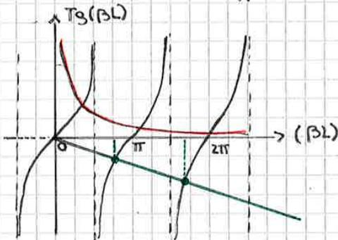
$$\begin{bmatrix} I_1 \omega^2 & G\beta \\ -G\beta \sin(\beta l) - I_2 \omega^2 \cos(\beta l) & G\beta \cos(\beta l) - I_2 \omega^2 \sin(\beta l) \end{bmatrix} \begin{Bmatrix} C \\ D \end{Bmatrix} = \begin{Bmatrix} 0 \\ 0 \end{Bmatrix}, \begin{Bmatrix} C \\ D \end{Bmatrix} = 0 \text{ TRIVIAL S.}$$
