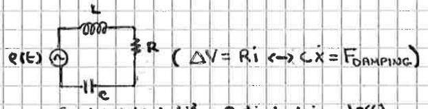
VOLTAGE KIRCHOFF LAWS  $\left\{ \begin{array}{l} \text{1st LAW: } L \frac{d^2 i}{dt^2} + R \frac{di}{dt} + \frac{1}{C} i = \frac{de(t)}{dt} \\ \dots \end{array} \right.$
