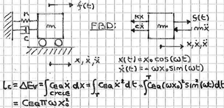
$$\alpha X_0^2 = c e a \pi \omega x_0^2 \Rightarrow c e a = \frac{\alpha}{\pi \omega} = \frac{h}{\omega} \quad h = \frac{\alpha}{\pi}$$
