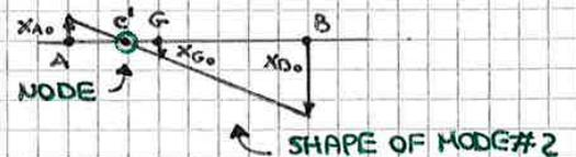
**NOTE:** MODE #1 AND MODE #2 ARE SYNCHRONOUS; THE SOLUTIONS REPRESENTED BY THESE 2 MODES ARE BOTH POSSIBLE SYNCHR. SOLUTIONS; SINCE THE S. IS LINEAR  $\rightarrow$  SUPERPOS. OF EFFECTS!
