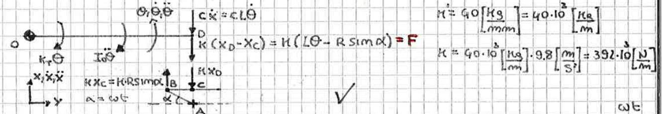
$$I_0 \ddot{\theta} + L^2 \ddot{\alpha} + L \cdot K (\theta - R \sin \alpha) + K_t \theta = 0 \leftrightarrow I_0 \ddot{\theta} + L^2 \ddot{\alpha} + (L^2 K + K_t) \theta = LKR \sin \alpha$$
