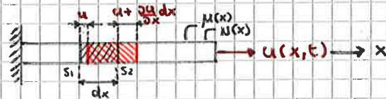
FBD:  $\mu dx \frac{\partial^2 u}{\partial t^2}$  (INERTIAL FORCE)
