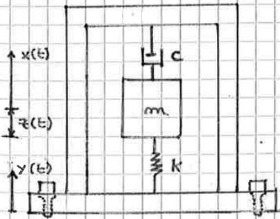
USED FOR MEASURING DISPLACEMENT AND ACCELERATION
