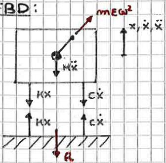
$$M\ddot{x} + C\dot{x} + Kx = m\omega^2 R \sin(\omega t) = m\omega^2 R e^{i\omega t} = \left(\frac{\omega}{\omega_m}\right)^2 m\omega_m^2 R e^{i\omega t} = f$$
