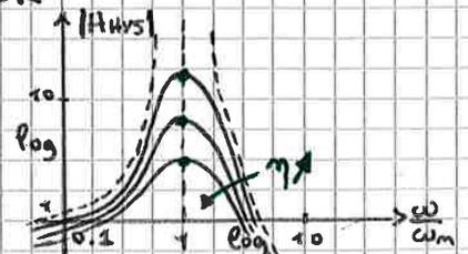
$c_{eq} = \frac{\alpha}{\pi \omega} = \frac{h}{\omega} = \frac{\eta k}{\omega}$  ;  $\omega = \omega_n \Rightarrow c_{eq} = \eta \cdot \frac{k}{\omega_n} = \eta \frac{\omega_n m}{\sqrt{\frac{k}{m}}} = \eta \omega_n m = \eta \sqrt{\frac{k}{m}} m = \eta \sqrt{k m}$
