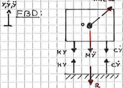
ENGINE STATIC UNBALANCE  $\times G = E\omega$
