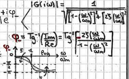
IN CASE OF UNDAMPED SYSTEM ( $\zeta = 0$ ):
