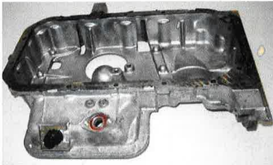
Simple oil pan in Al-alloy and double steel sheet (Isuzu 1.1 CDTI)
