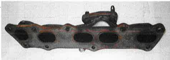
Sheet steel exhaust manifold (Honda 2.2 i-CTDi)
