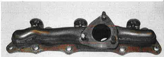
Cast iron exhaust manifold with turbocharger (VW 2.0 TDI)
