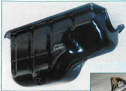
Simple oil pan in steel sheet (FIAT Fire 8v)
