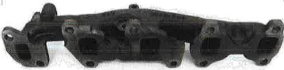
Cast iron exhaust manifold (FIAT SDE 1.3 16v)
