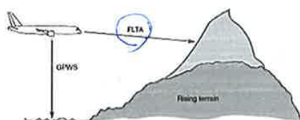
TAWS - Terrain Awareness Warning System GPWS - Ground Proximity Warning System FLTA - Forward Looking Terrain Awareness
