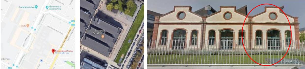
We used a Total Station to acquire the coordinates (with respect to our relative position) of 3 points having a prism reflector called 101,102,103. Then, changing the settings of acquisition type to NP (non prism), we acquired natural points belonging to the facade. There were some points marked by us with a paper and other corner points belonging to the facade's elements.
