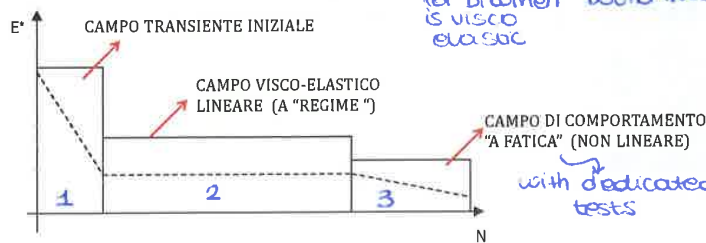
Mechanical response as a function of increasing cyclic loadings.
