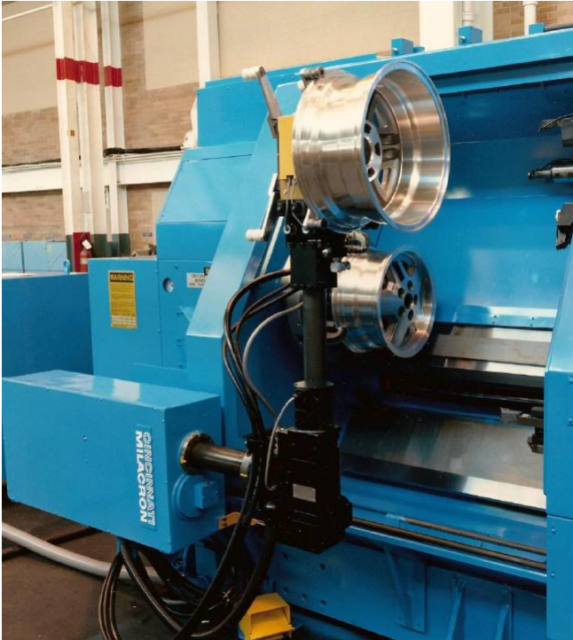
A robotic arm performs unloading and loading operations in a turning center using a dual gripper.
