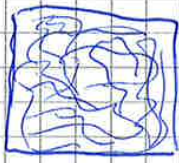
cracks without reinforcement
