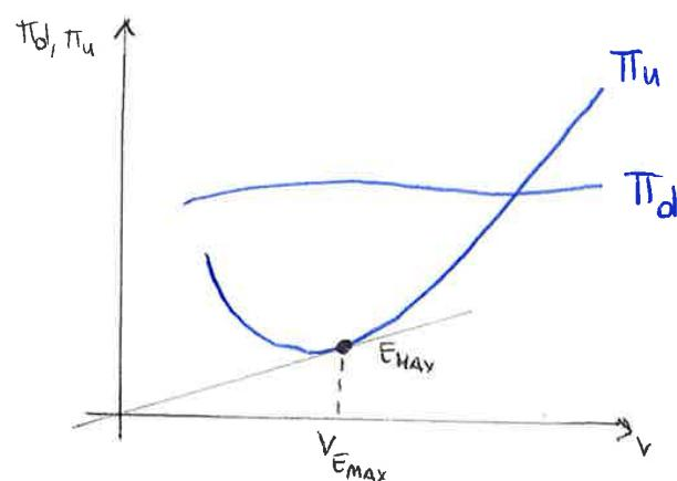
$$\begin{cases} C_{L(E_{MAX})} = \sqrt{\frac{C_D}{K}} = \sqrt{\frac{0,02}{0,044}} = 0,674 \\ C_D(E_{MAX}) = 2 C_{D0} = 0,04 \end{cases}$$
