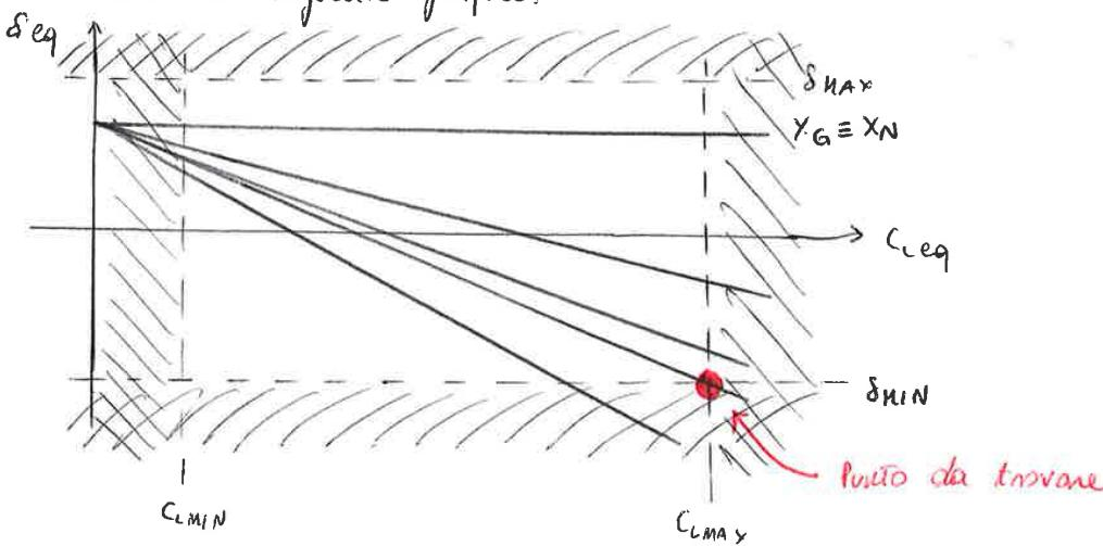
$$\begin{cases} C_{L\text{eq}} = C_{L\alpha} \cdot \delta_{\text{eq}} + C_{L\delta} \delta_{\text{eq}} \\ C_{H\alpha} = C_{H0} + C_{H\alpha} \cdot \delta_{\text{eq}} + C_{H\delta} \delta_{\text{eq}} \end{cases}$$
