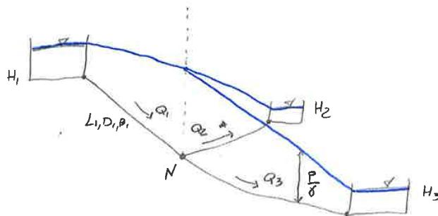
$$\left. \begin{array}{l} L=3 \\ n=1 \end{array} \right\} 4 \text{ incognite} \\ (Q_1, Q_2, Q_3, H_N) = ?$$
