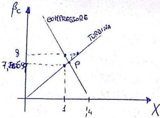
$$\frac{1+\alpha}{\alpha} \cdot \dot{m}_a \frac{\sqrt{RT_3'}}{P_3'} = \frac{1+\alpha}{\alpha} \cdot \dot{m}_{a0} \frac{\sqrt{RT_3}}{P_3}$$
