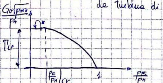
$\frac{G_{LP} \sqrt{p_{H'}^* v_{H^*}^*}}{p_{H^*}} = \frac{G_{LP} \sqrt{p_{H'}^* v_{H^*}^*}}{p_{H^*}} = \Gamma_{LP}^*$
